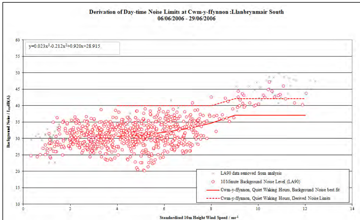
Figure 9.6 Background Noise Levels and derived limits During Quiet Waking Hours at Cwm-y-ffynnon
