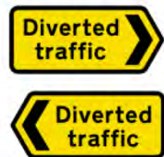
TSRGD DIAG. 2704 DIRECTION OF TEMPORARY DIVERSION ROUTE.
