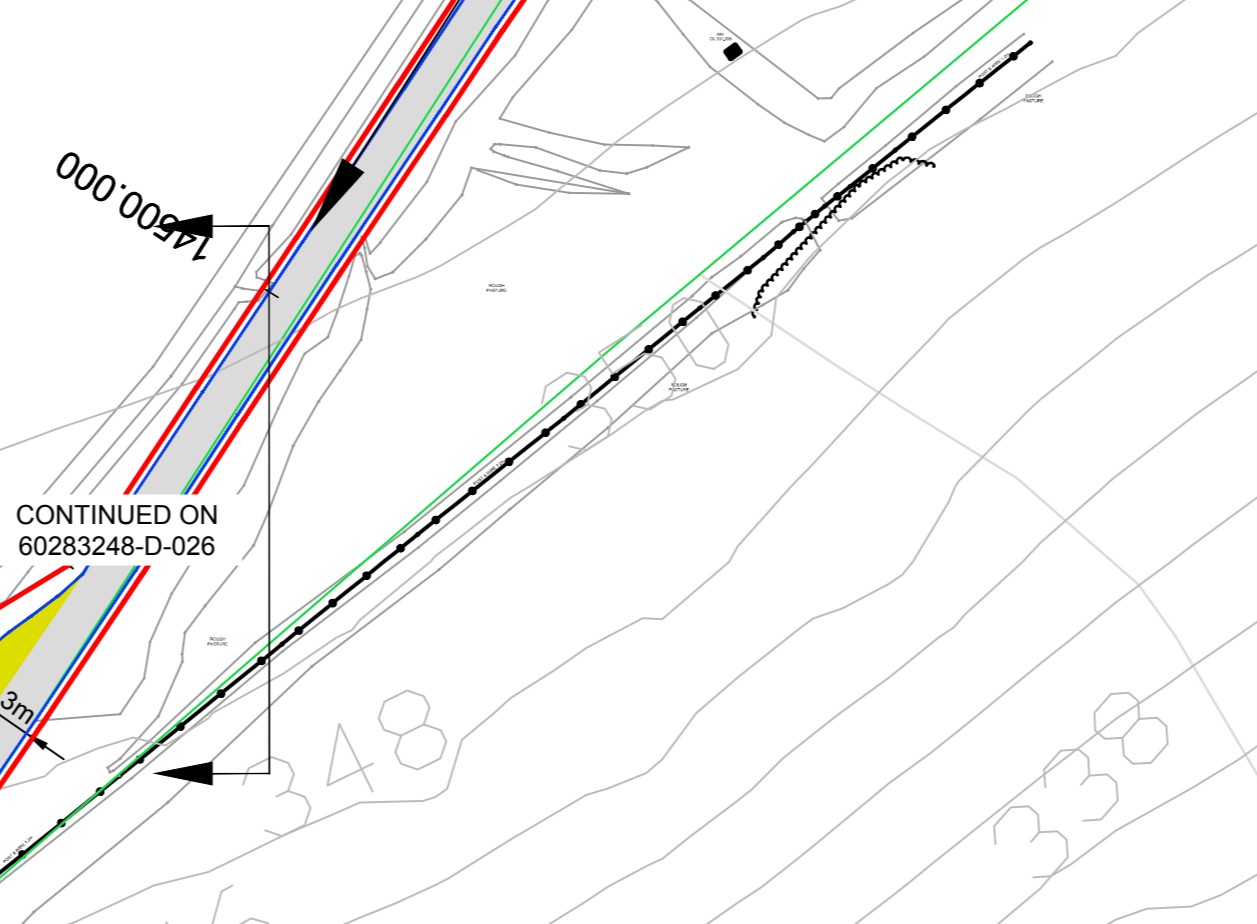
3.7 - EXISTING PASSING AREA AT CATTLE GRID CH 14200 EXISTING UNBOUND PASSING PLACES ARE LOCATED ON EITHER SIDE OF THE EXISTING CATTLE GRID. ALTHOUGH THESE AREAS ARE OF INSUFFICIENT SIZE TO ACCOMMODATE A WAITING HGV, EXISTING INFRASTRUCTURE TO BE RETAINED FOR USE BY GENERAL CONSTRUCTION VEHICLES.
